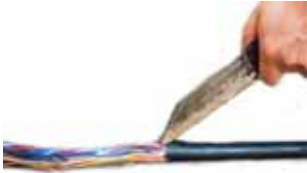
Prepared the cable, cut and remove cable sheath.
